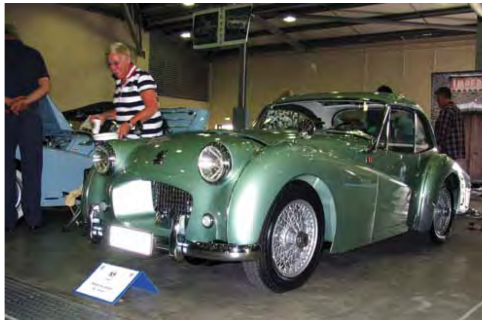
All the TRs that were shown at Harrogate were in one of the huge buildings for the Fairgrounds. In the Masters Class is the TR2 Francourchamp belonging to Patrick Van Houtven from Belgium where these unique cars were built. Notice in the side view that due to the rigid roof, that the door is lengthened for easier entry and the rear dogleg (quarterpanel) has been trimmed. The windows crank up and down with a simple crank and bicycle chain guides on sprockets. Since all the TRs assembled from kits in Europe were sprayed there, the colour, in many cases was not the same as the cars assembled in Coventry.
